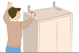
Fix cupboard doors and so on with fastening plates.
